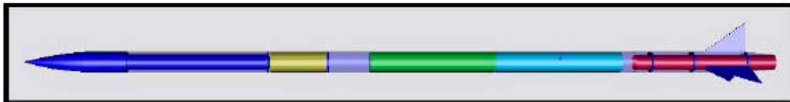
Figure 2: 3D Model. Color code: blue – structural elements, red – propulsion, cyan – cold temperature payload compartment, green – ambient temperature payload compartment, yellow – electronics bay. The drogue parachute is housed below the electronic bay, the main parachute is above the electronic bay.
